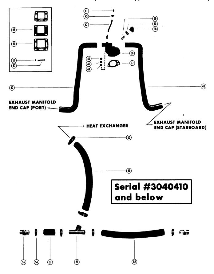
FRESH WATER COOLING KIT (MARINE 215)(TO HEAT EXCHANGE)
