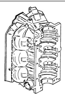
Chrome cylinder bores which are damaged or are scored can be rechromed to the original dimensions. U.S. Chrome Corporation of Wisconsin offers this service. Any question concerning the repairability of a block should be referred to the attention of the service manager at U.S. Chrome.
