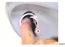
a - Inner end of tilt pin spiral retaining ring
