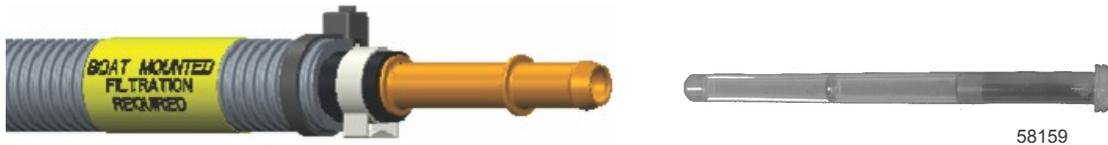
4. A fuel demand valve (FDV) is no longer required on the fuel supply hose. The vent and purge valves are not used with this fuel delivery system; therefore, a primer bulb can be utilized, if desired.
