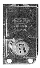
It has been brought to our attention that, occasionally, the external wiring hamess is not being plugged into the voltage regulator properly. This condition will show as a full charge on the ammeter at all times above half-throttle and eventually will cause damage to the battery.
