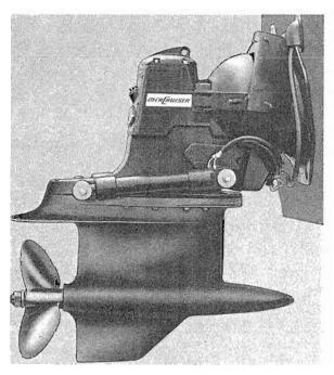
with these Super Speedmaster units as a package (less propeller). (Figure on left) The package will be equipped with the Heavy Duty Power Trim (B-39881A2), which was listed in the same Service Bulletin. The Heavy Duty Power Trim permits easy trimming of the boat for fast planing of heavily loaded boats and to maintain an even "plane" in rough water when operating at cruising speed.
