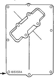
"A" after Number Designates a Lower Pressure Pump to Be Used for Replacement of the Small Reservoir White Pump
