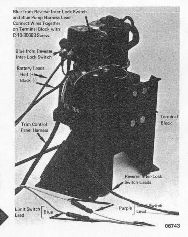
WARNING: Operation of an incorrectly wired pump may result in damage to pump, reverse lock valve, trim cylinders, wiring and/or trim system connecting hoses and lines.
