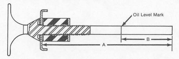
The approximate distance from end of dipstick to the underside of the cap (dimension "A") and from end of dipstick to the oil level mark (dimension "B") are charted below. These dimensions will help identify each dipstick.
