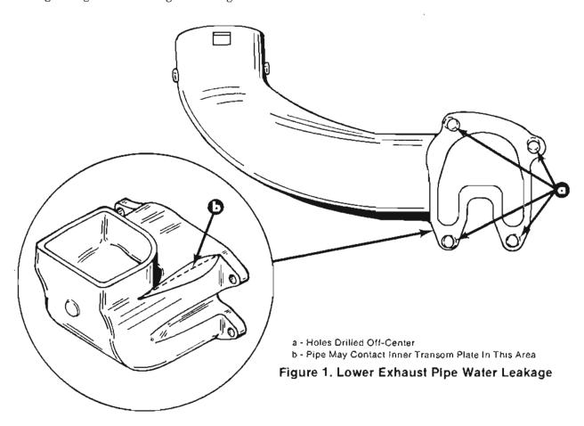
If you encounter a power package with either of the above conditions, install new, lower exhaust pipe, 42421A5. Labor allowance is 3.5 hours.
