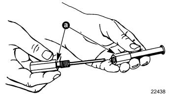
a - Swivel Bushing Removal Tool (Snap on CG40A6 and CG40-4)
