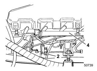
1990 V6/V8 Stern Drive and Inboard engines built after October 1, 1989 will not have exhaust manifold water drain petcocks. The drilled and tapped hole in the manifold (for the petcocks) has been eliminated.
