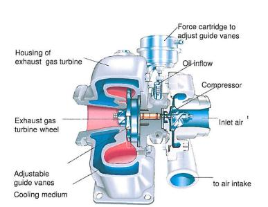
Installation of exhaust gas turbochargers with improved corrosion behaviour.
