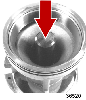
Pressing the outer propeller shaft seal from the bearing carrier
