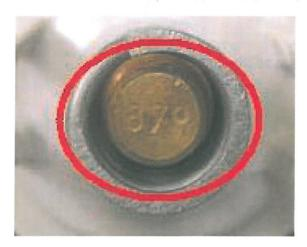
Step 7 - Reinstall thermostat and tighten screws to 10 Nm.
