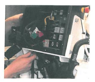
Step 3 – Disconnect the harnessing from the electrical box
