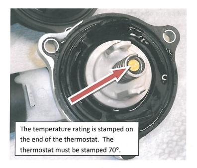
If the thermostat is stamped 87°, then the thermostat assembly must be replaced, P/N 06V 121 111.
