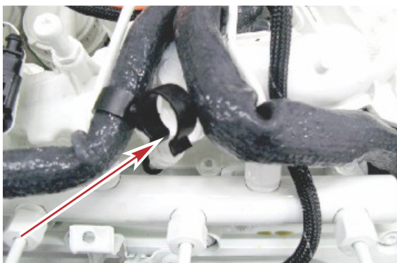
Remove the fuel lines from the retainer
