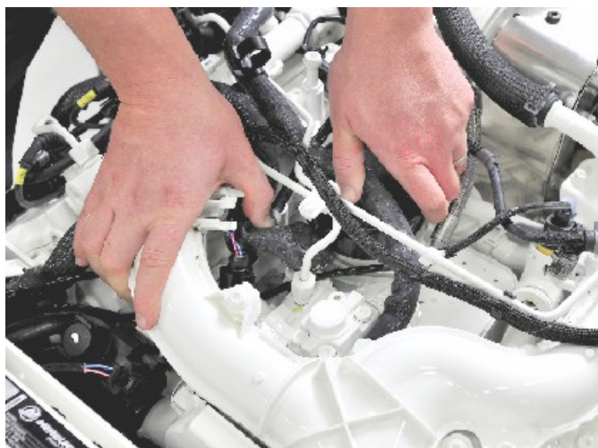
Spread the fuel lines apart to gain access to the oil supply line
