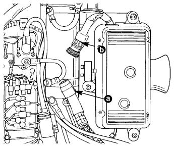
a - Engine Connector b - ECU Connector
