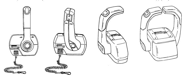
2. **Determine if your Commander 3000 control is included in this recall.** View the decals on the control, if visually accessible, in the location shown below. Use a flashlight and mirror to help read the decals.
