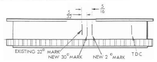
In order to accurately time the engines with the old style flywheels, it is necessary to add the timing marks for 28° and 30°. These marks are added by simply scribing one line 5/32 of an inch to the right of the 32° line and another line 5/16 of an inch to the right of the 32° line. See Figure 2.
