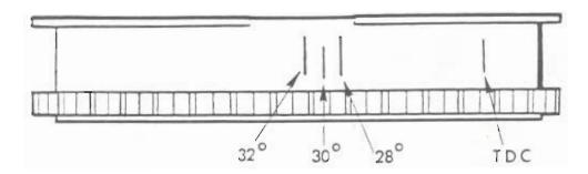
Older production flywheels may not have all the markings as indicated in Figure 1. The older flywheels are marked as in Figure 2.
