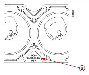
a - Casting number on bottom side of flange
