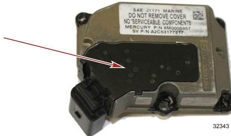
Newer style boost-by-pass valve has a black plastic molded insert.
