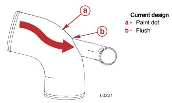
Exhaust elbows with the current design idle relief tube can be identified by a white paint dot on the top of the idle relief tube.
