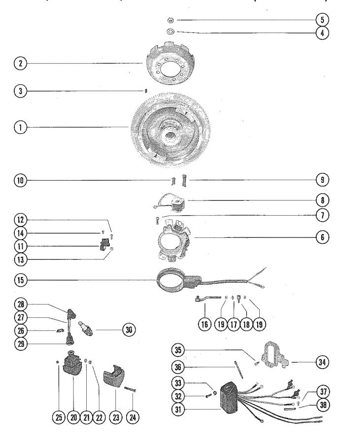
FLYWHEEL, IGNITION COIL, STATOR AND SWITCH BOX(GROUP NO. 15)
