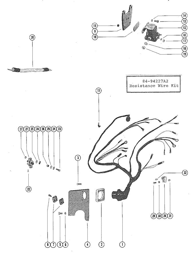
WIRING HARNESS, CIRCUIT BREAKER AND STARTER SOLENOID (STERN
