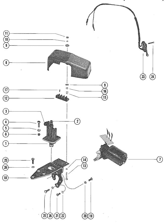
REVERSE LOCK VALVE AND SHIFT ACTUATOR (STERN DRIVE)
