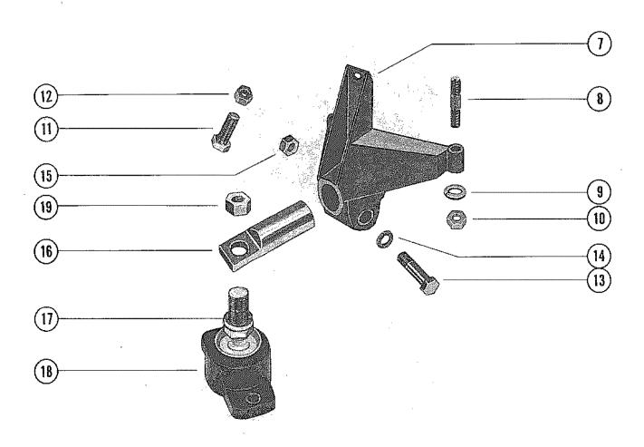
TRANSMISSION AND ENGINE MOUNTING (INBOARD)
