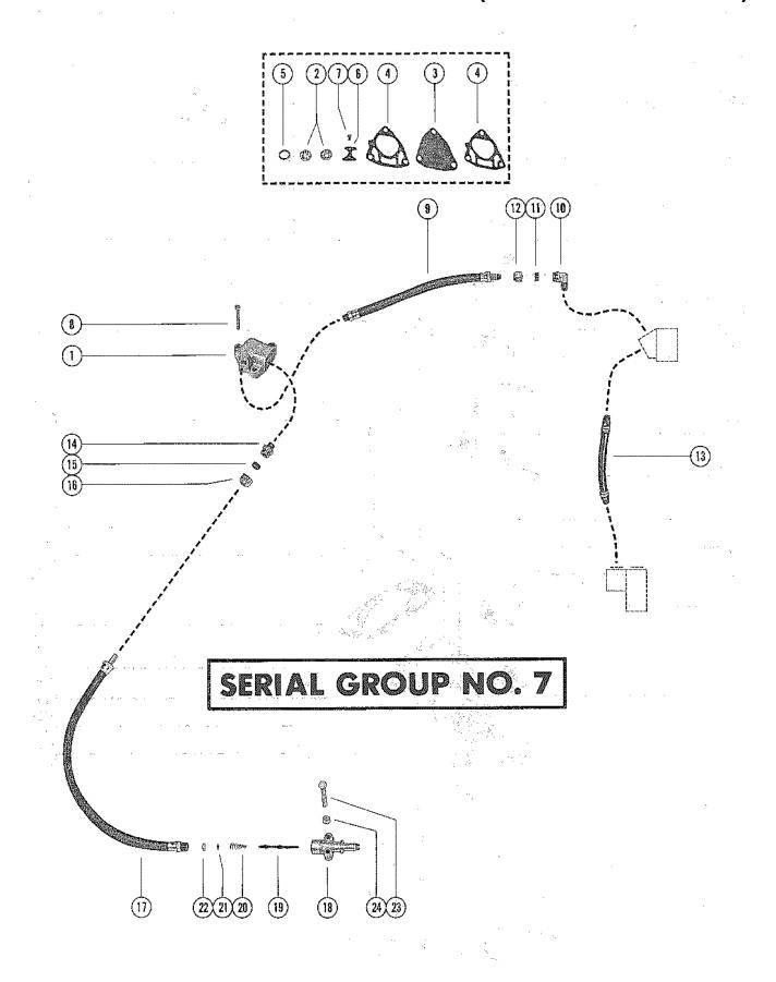
FUEL PUMP AND FUEL LINE ASSEMBLY (SERIAL GROUP NO. 7)
