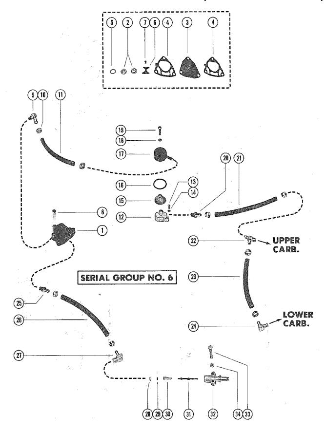
FUEL PUMP AND FUEL LINE ASSEMBLY (SERIAL GROUP NO. 6)
